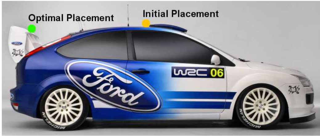
Figure 3.6: Initial and Optimal magnetometer placement (Original photo courtesy of www.fordteamrs.com )
