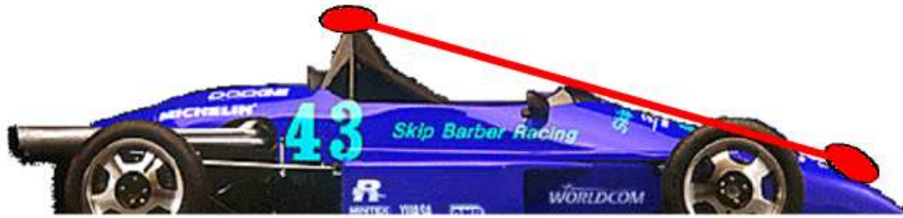
Figure 2.6: Multiple GPS antennae mounting on racecars[3]
