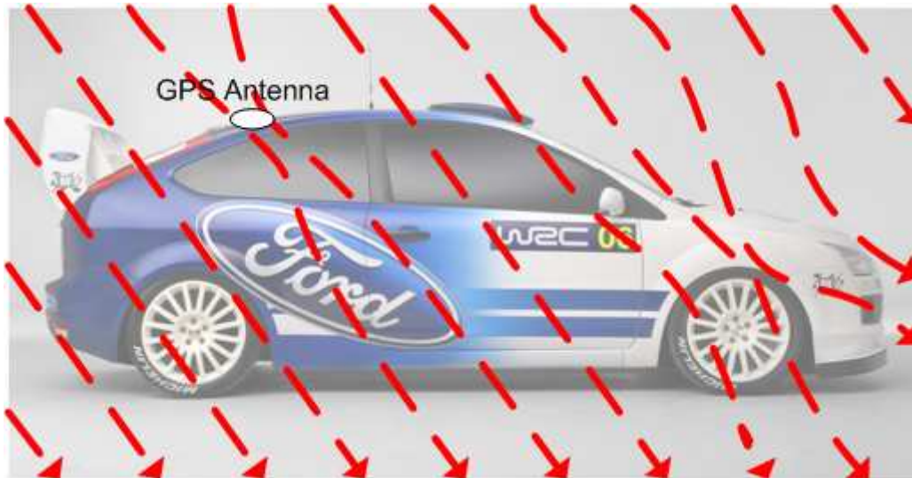
Figure 3.5: Magnetic field distortion due to Engine and GPS Antenna (Original photo courtesy of www.fordteamrs.com )
