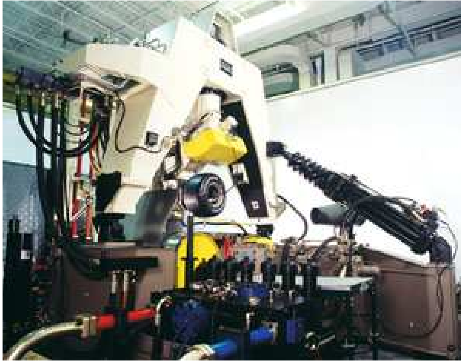
Figure 2.9: Bridgestone's MTS Flat-Trac Tyre Testing System[5]
