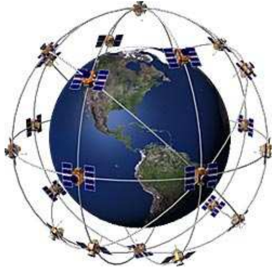
Figure 2.3: GPS Satellite Orbits (courtesy of www.garmin.com )
