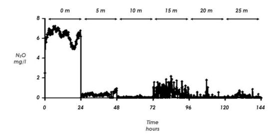
Figure 11: N<sub>2</sub>O aeration lane profile results at Finham
