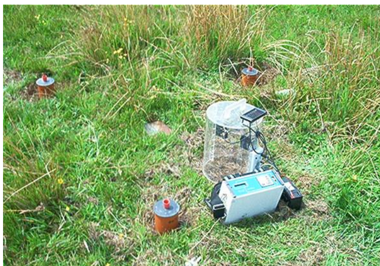
Figure 52: Closed chamber systems for monitoring CO 2 evolution from below ground.
