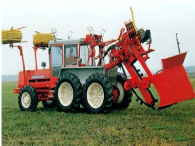
Figure 39: Conventional commercial machinery for installation of slotted plastic pipe.
