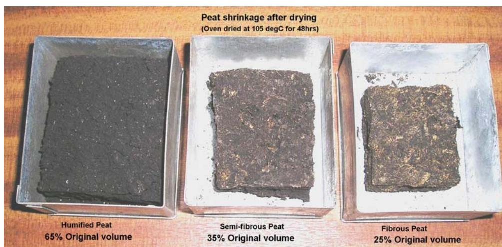
Figure 20: Shrinkage of 3 different peat types from Methwold Fen.
