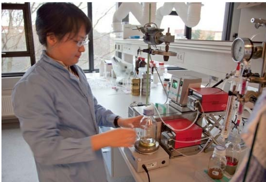
Figure 7.3: The former PhD student Yuan Xu is producing Biodiesel in a Batch Reactor
