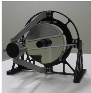
Fig. 2. Photograph of the assembled Ritchey-Chrétien Telescope with 10 cm of aperture.
