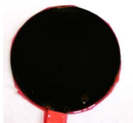
Figure 4: Platinum black surface electroplated at DTU
