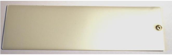
Figure 6 Nickel plate coated with approx. 20 \mu\text{m} of aluminium via Magnetron sputtering is a plasma vapour deposition
