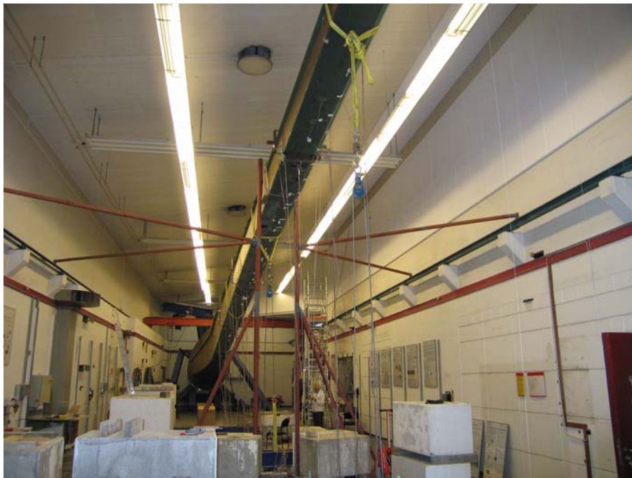
Figure 56: A view of the test setup from the tip of the girder. The guides is the brown columns in the middle of the picture.
