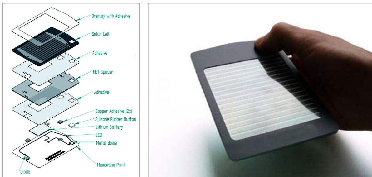
Figure 30: The lamp produced according to principle 2, exploded view to the right, from (Krebs F. C., Fyenbo J., Jørgensen M., 2010)
