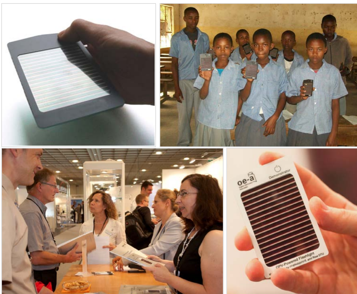
Figure 42: The two LED torches demonstrated: the reading lamp for school children (top) and the “easy-to-carry-with-you” torch targeted at the western market.
