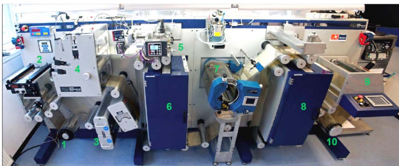
Figure 7: In-line printer comprising unwinder (1), edge guide/slicer (2), double-sided cleaner (3), flexographic printer (4), slot-die coater (5), oven (6), rotary screen printer (7), oven (8), cutter (9) and rewinder (10).
