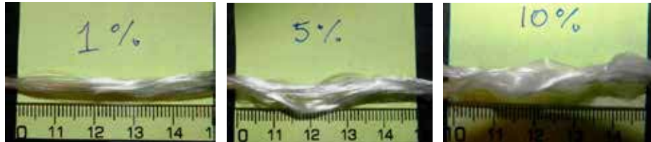
Fig. 2. Glass/LPET fibre yarns with three levels of “overfeed”.
