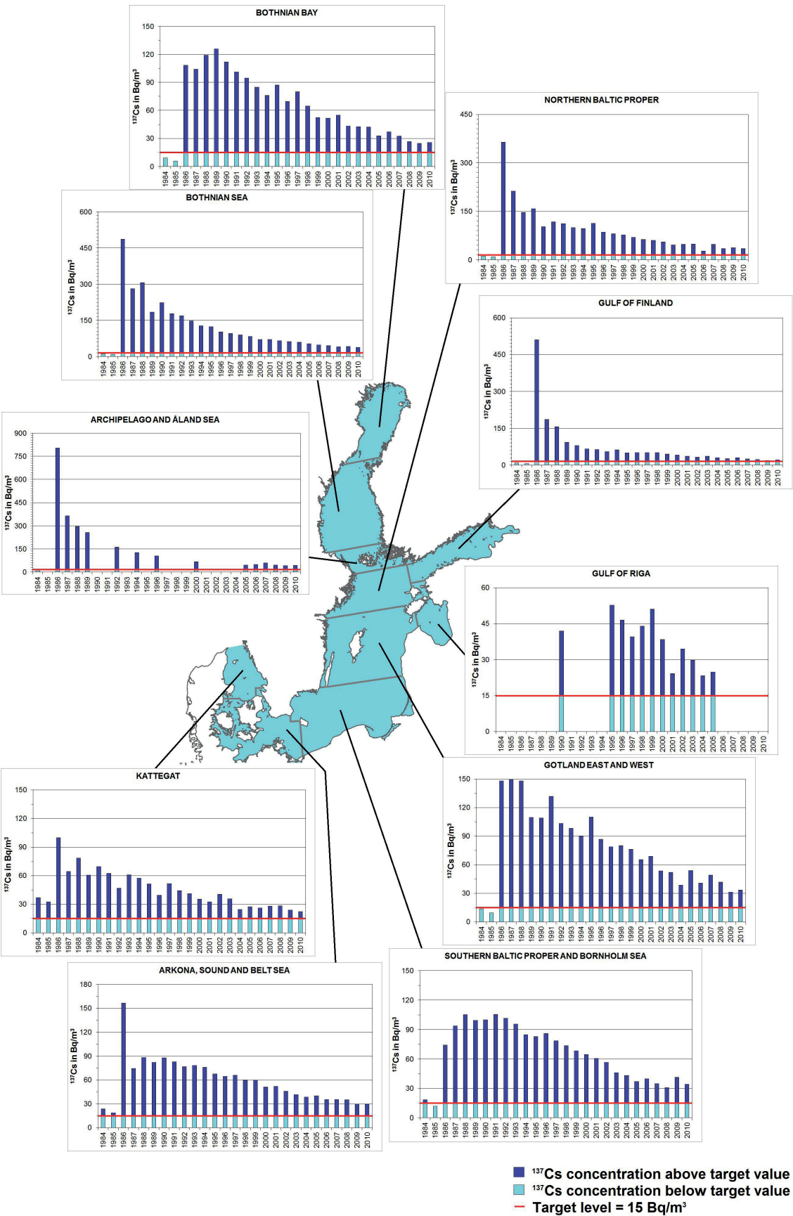
Figure 3a.1. ^{137}\text{Cs} concentrations (Bq/m 3 ) in surface water (sampling depth \leq 10\text{m} ) in 1984-2010, as annual mean values by basin. Target values have been calculated as the average of pre-Chernobyl (1984-1985) concentrations.
