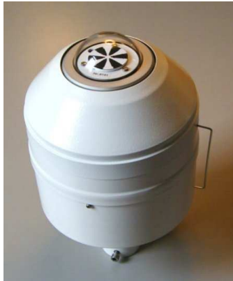
FIGURE 4.2: A pyranometer of the type Star pyranometer by Phillip Schenk
