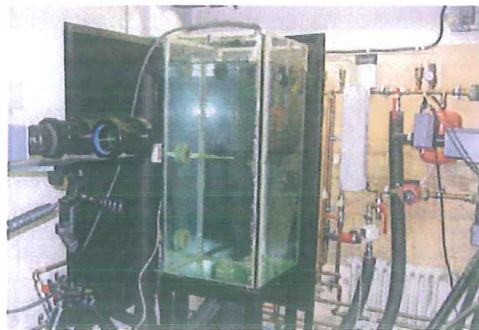
Fig. 1. The PIV test facility of the smart solar tank with one heating element and a side-arm.
