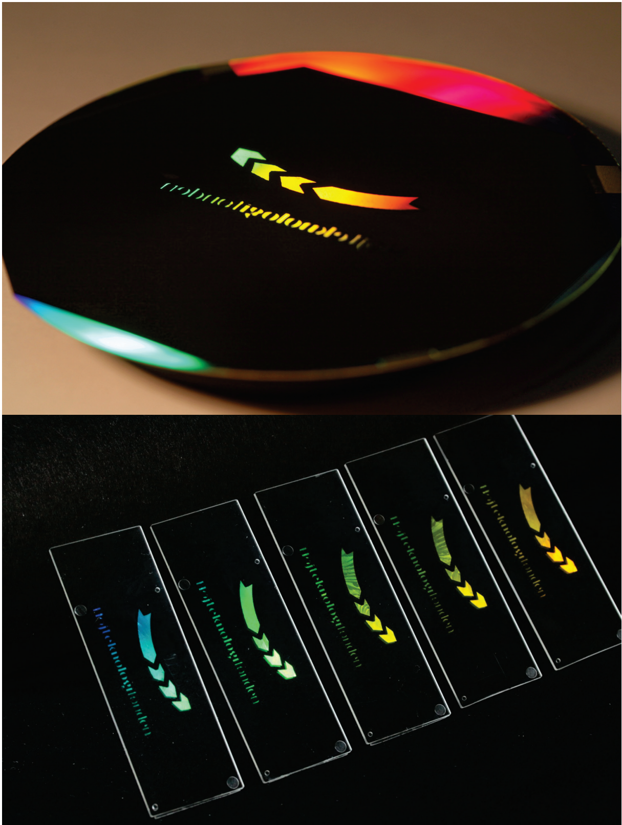
Figure 7. Photo of a Ni tool with nanopattern only on the area not shielded by a laser cut shadow mask (top) and photo of injection molded polymer microscope slides, created using the same tool, showing logo of The Danish National Advanced Technology Foundation (bottom).
