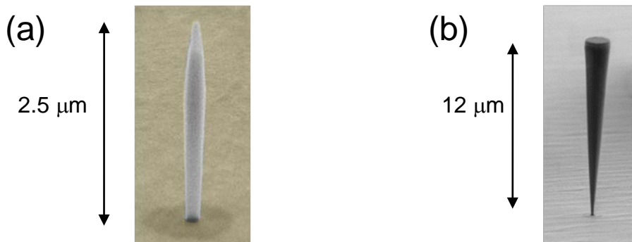
Fig. 2. Scanning electron micrographs of photonic nanowires implementing a regular conical tapering (a) and an inverted conical “trumpet” tapering (b).
