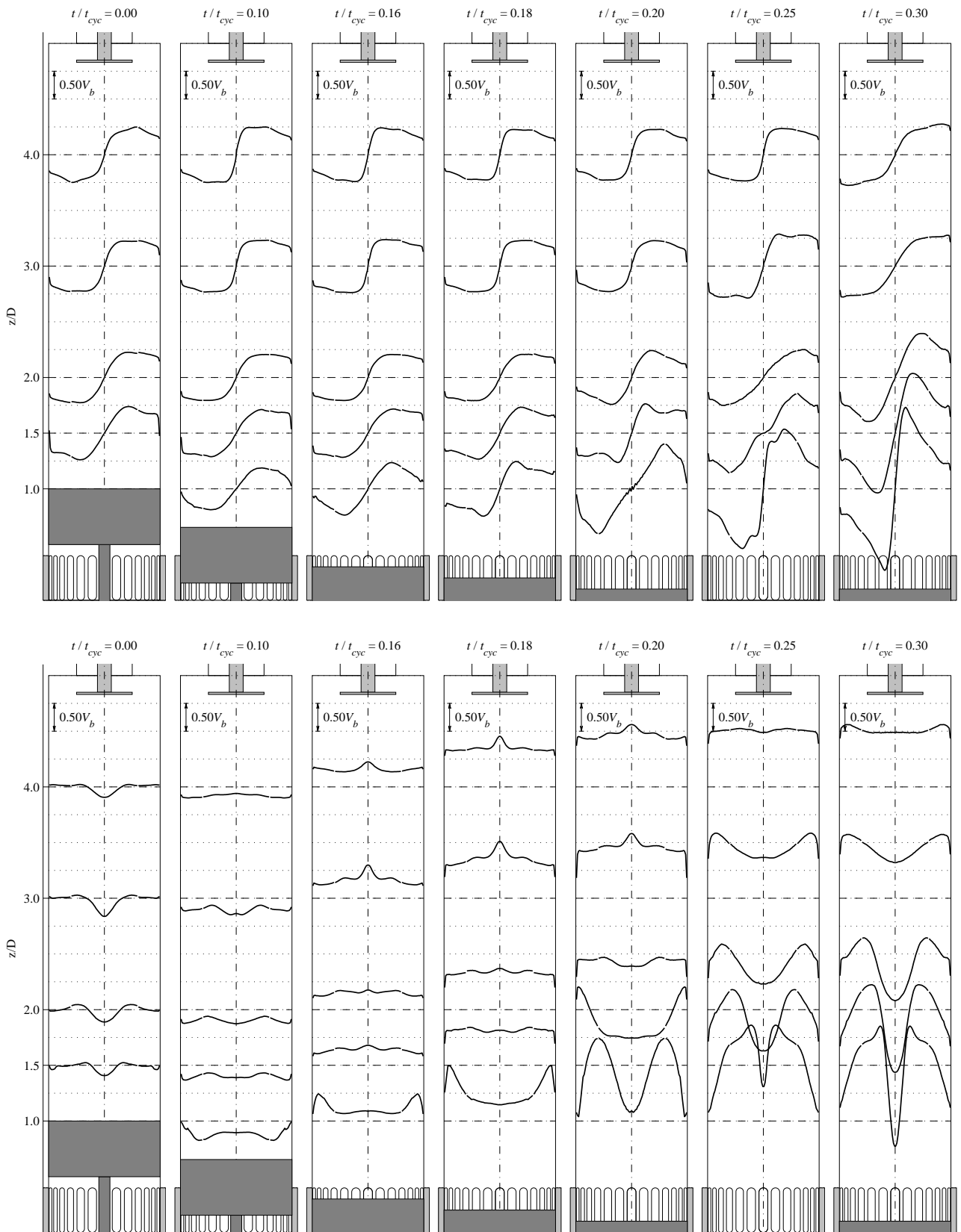
Figure 7: Radial profiles of phase-averaged velocity for different times during the cycle. ( top row ) Tangential velocity V_\theta/V_b , ( bottom row ) axial velocity V_z/V_b . The figure is continued on Figure 8.
