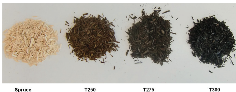
Fig. 1 – Color change during the torrefaction process. (For interpretation of the references to colour in this figure legend, the reader is referred to the web version of this article.)
