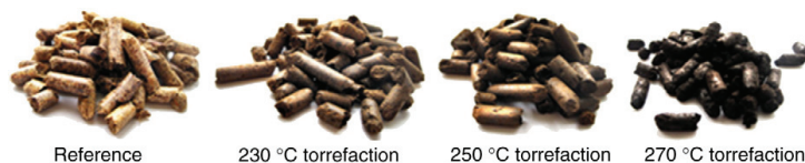
Fig. 2. Images of untreated Scots pine pellets and pellets torrefied at different temperatures for 1 h.
