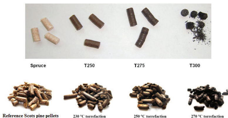
Figure 14: Images of pellets made from torrefied spruce with residence time of ca. 2 h (paper III) and Scots pine pellets that torrefied subsequent to pelletization for about 1 h (paper IV).
