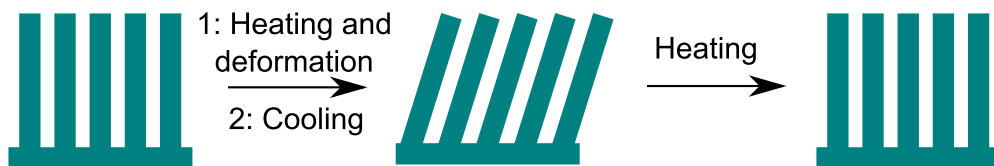
FIGURE 1.2: The principle behind the switchable adhesive prepared by del Campo et al.[11] The patterned surface exhibited adhesion. Upon heating and deformation of the fibrils a non-adhering state was obtained. The non-adhering state could be fixed by cooling. Heating the surface reformed the adhering state.
