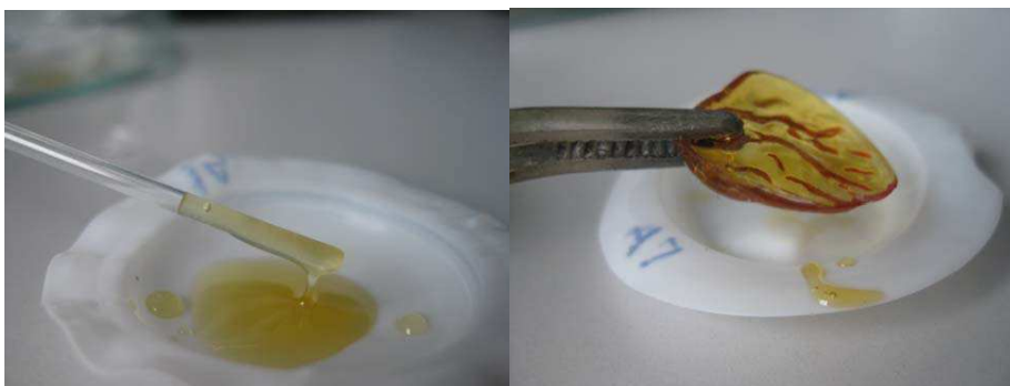
Figure 7: Film formation of P1 after UV-irradiation. A) P1 before UV-irradiation. The material is a liquid. B) P1 after 96 h of UV-irradiation. The material is cross-linked to a film.
