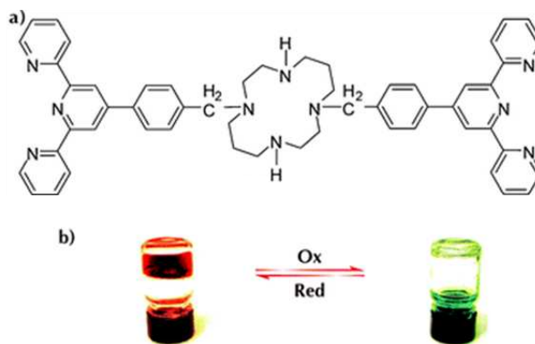
FIGURE 2.11: a) Two terpyridine groups linked with a cyclam (1,4,8,11-tetraazocyclotetradecane) macrocycle. b) Addition and complexation with \text{Co}^{+2} yields a red redox-responsive metallo-supramolecular polymer gel. The gel can be oxidized to a green sol. The red gel is restored by reduction. The redox-effect can be controlled electrochemically [54]. (Adapted and reprinted with permission from Langmuir , 25(15):8751–8762, 2009. Copyright (2009) American Chemical Society.)
