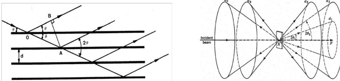
Figure 3.1. A simplified illustration of the phenomena behind Bragg-Brentano (left) and Debye-Scherrer (right) type diffractometers. (32).
