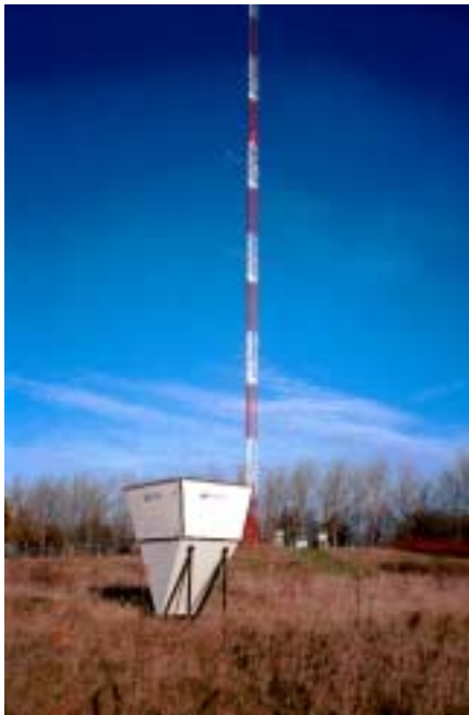
Figure 14 Comparison of sodar measurements with stationary mast (Re. Ioannis Antoniou, Risø)
