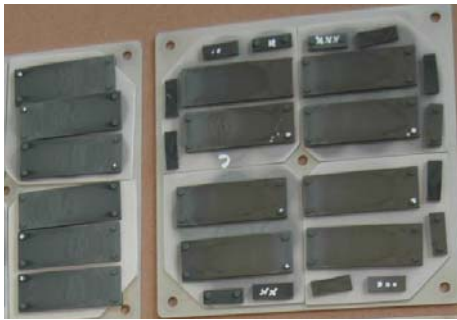
Figure 5: Injection moulded specimen with different moulding conditions.
