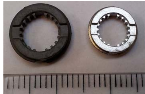
Figure 1: Example of moulded metallic parts (Green part-left, and Sintered final part- right)-courtesy of Sintex A/S, Denmark.
