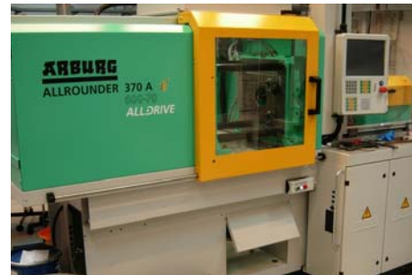
Figure 4: Injection moulding machine used for molding of the metal parts with the binder.
