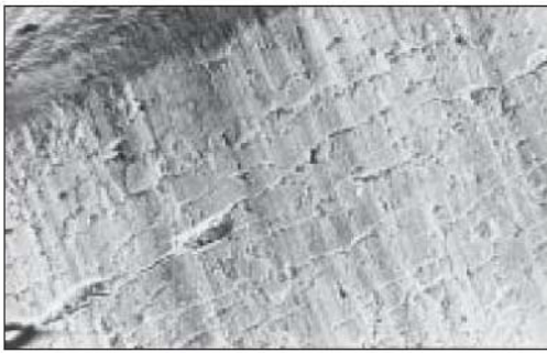
Fig. 3a: Adhesive wear [6]
