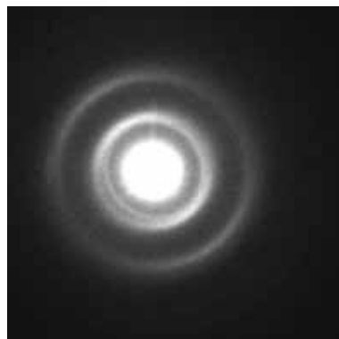
Figure 6.2: Uncalibrated TEM diffraction pattern taken from Au particle during dissolution. Misalignments in the imaging system likely led to the split rings seen. However, the presence of rings indicates polycrystallinity in the particle.
