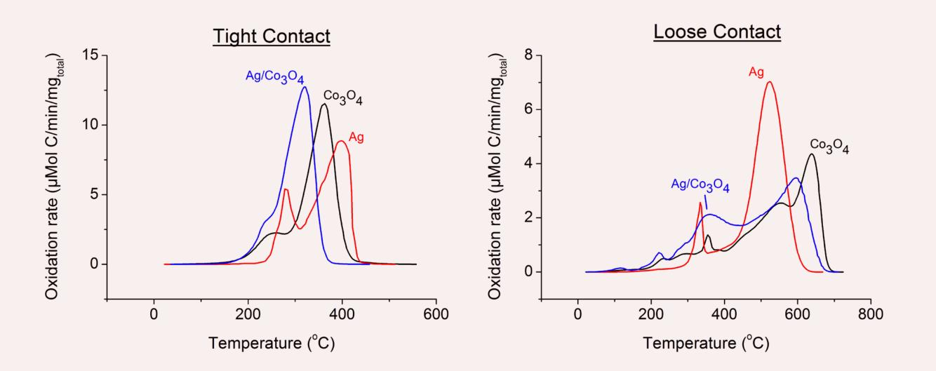
→ Performance of cosupported catalyst cannot be directly described in terms of the activity of the single Ag and Co<sub>3</sub>O<sub>4</sub> components
