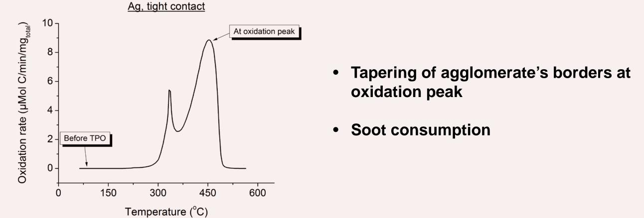
$\rightarrow$  Soot oxidation is an exothermic process. Local heating could lead to melting of the advancing Ag (seen on metal nanoparticles in literature [1] for graphite oxidation). Once oxidation is over, Ag could solidify again.
