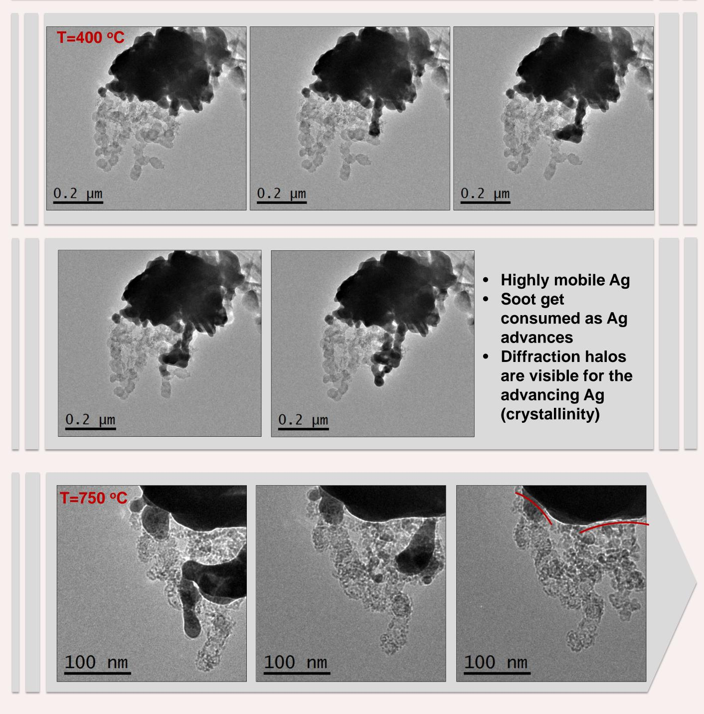
1 NL/min flow of 10 vol%  $O_2$  in  $N_2$ . 100 to 750 °C at a rate 11 °C/min.
