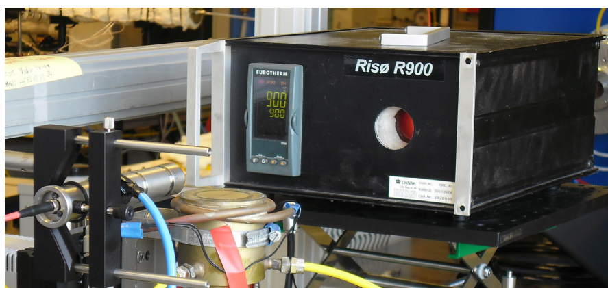
Figure 20. The blackbody radiation source. The temperature of the cavity was 894.4 °C (1167.6 K).
