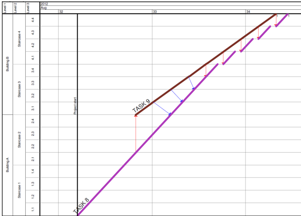
Figure 24: Layer 5 logic. Dependency across structural independent locations.
