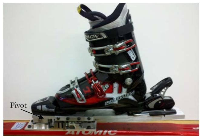
Figure 5. Group 3 final design [Austin et al. , 2011]. The pivot point is at the toe of the plate device. The plate rotates downward at the heel about this point.
