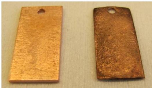
Figure 3.3: Cu electrode as received (left) and Cu electrode covered with nanoparticles (right).
