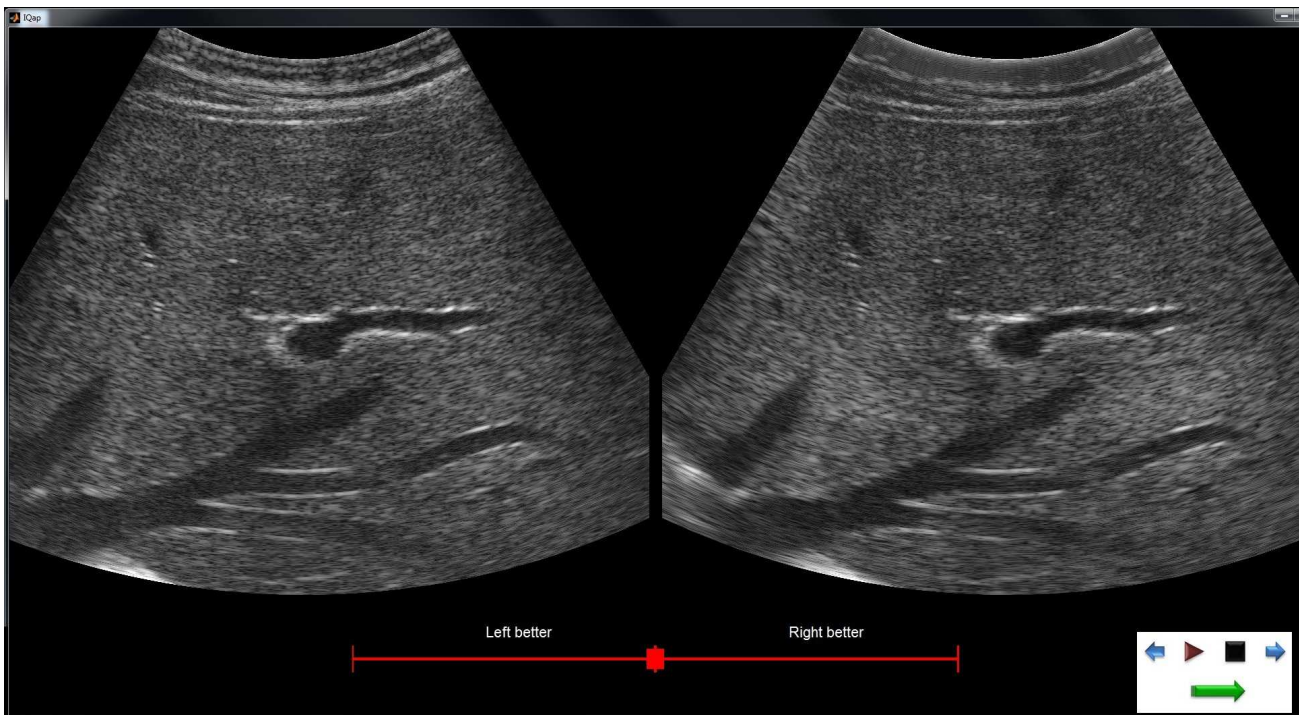
Figure 2. Visualization of an image pair for overall image quality evaluation. The VAS is shown in the bottom and the control panel for navigating the sequences are shown in the lower right corner. In this case, DRF-THI is shown on the left and SASB-THI is shown on the right.
