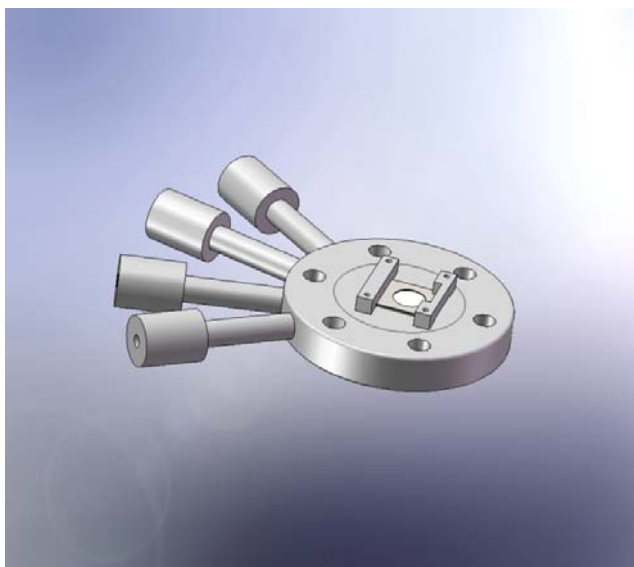
Fig. 5.10 An open \mu -reactor mounted on the manifold block obtained from a 2 \frac{3}{4} inch stainless steel flange for UHV application.
