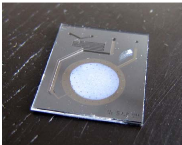
Fig. 2.2 Anodically bonded \mu -reactor loaded with catalyst.
