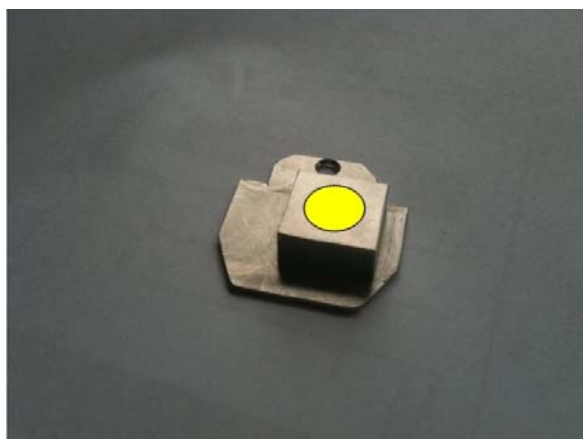
Fig. 5.11 Metallic frame sample holder that is used to seal the open \mu -reactor. The area where the catalyst should be deposited is colored in yellow.
