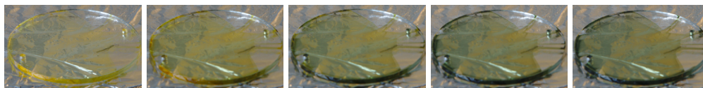
Figure 4.1.: The spin coated reaction mixture polymerises on a hot plate forming the conductive polymer PEDOT. The pictures were taken at approximately one minute intervals.
