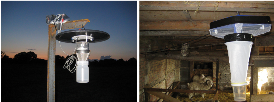
Figure 2.2: Two widely used trap types for Culicoides : The CDC mini trap type with a 4 W light tube hung in a heavy metal gallows on a field with sheep (left); and the Onderstepoort type with an 8 W light tube hung in a goat stable (right).
