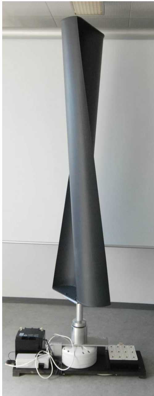
Figure 57 – Lab model of the energy system for the designed hybrid street lighting system
