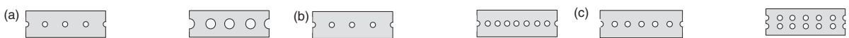
Fig. 6 Hybrid-bearing parameters configurations. (a) Hybrid-bearing parameters: orifice diameter. (b) Hybrid-bearing parameters: orifices in circumferential direction. (c) Hybrid-bearing parameters: orifices in circumferential direction
