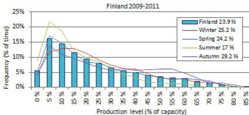
Figure 13. Frequency distributions of wind power production in Finland during 2009–2011.
