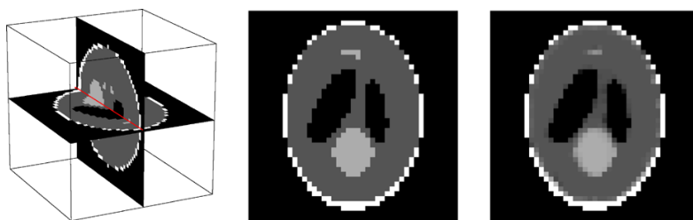
Fig. 2 Left : Two orthogonal slices through the 3D Shepp-Logan phantom discretized on a 43^3 grid used in our test problems. Middle : Central horizontal slice. Right : Example of solution for \alpha = 1 and \tau = 10^{-4} . A less smooth solution can be obtained using a smaller \alpha . Original voxel/pixel values are 0.0, 0.2, 0.3 and 1.0. Color range in display is set to [0.1, 0.4] for better contrast
