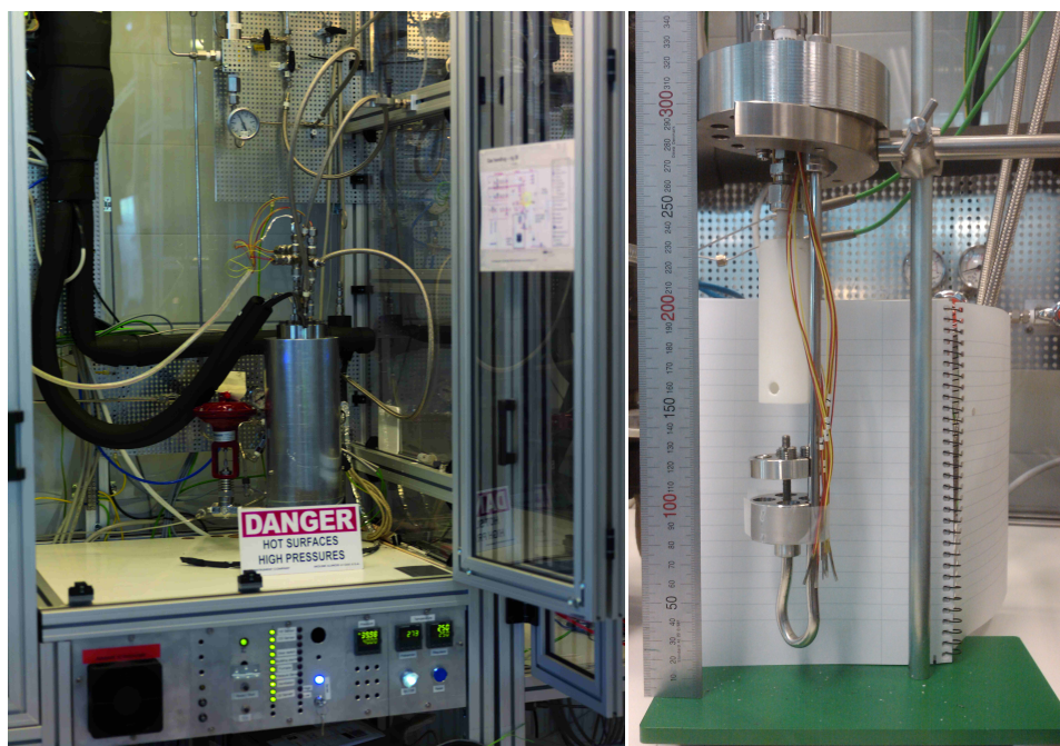
Figure 6.3: Picture of the autoclave in the automated test setup (left), picture of the sampleholder and holder for the catalytic burner (white ceramic body) (right).
