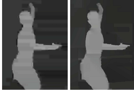
Fig. 4. Details of reconstructed depth images from the “ballet” data set [6]: standard H.264/AVC Intra (left) and plane fitting exploiting color segmentation (right), both at 0.025 bpp.
