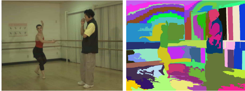
Fig. 3. Compressed color data (left) and relative segmentation (right) used to predict shapes in the depth image.
