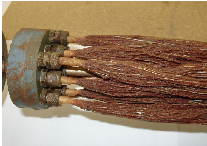
Figure 7: Pressure header of a hollow fibre MABR module
