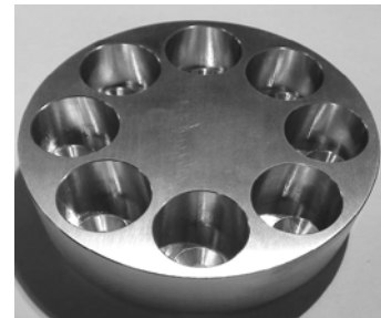
Figure 21: Piston crown with eight cylindrical chambers
