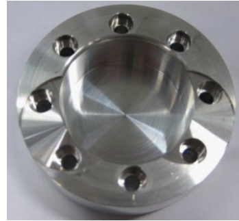
Figure 17: Diesel bowl piston crown
