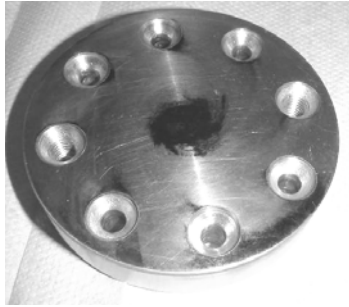
Figure 16: Flat piston crown
