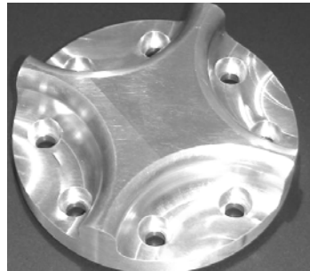
Figure 19: Piston crown with four side chambers
