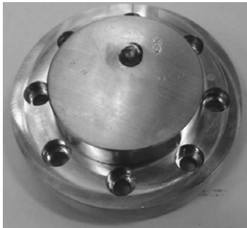
Figure 18: Piston crown with ring shaped chamber
