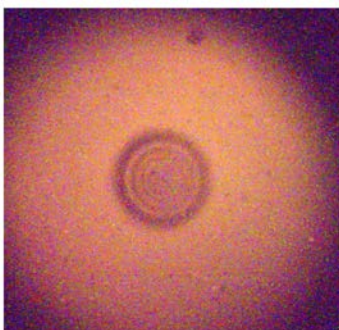
Fig. 10. Polarization microscope picture of the area irradiated at 670 nm. The film is at 45° to the polarization direction.
