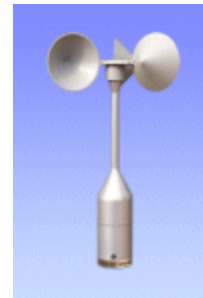
The Risø P2546 cup anemometer
