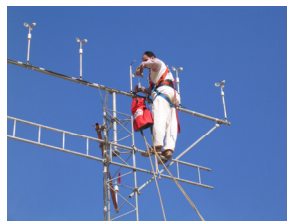
10 anemometers being calibrated – reference anemometer in middle position: ○
