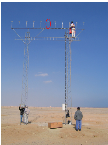
10 anemometers being calibrated – reference anemometer in middle position: ○
