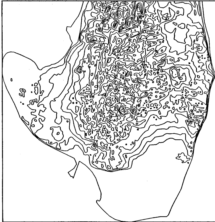
Figure 27. Example of the height contours obtained by digitizing a standard topographical map, cf Fig. 26.
