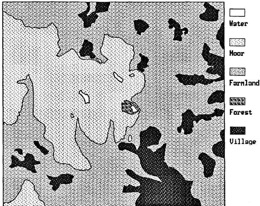
Figure 20. Example of a roughness map obtained by digitizing the roughness-change lines on a standard topographical map.
