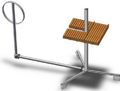
Figure 1 Principle test setup of 1kW DeepWind demonstrator wind turbine
