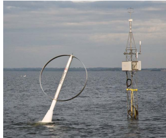
Figure 9 DeepWind demonstrator in operation and tilting towards mast with medium wind from south and low waves
