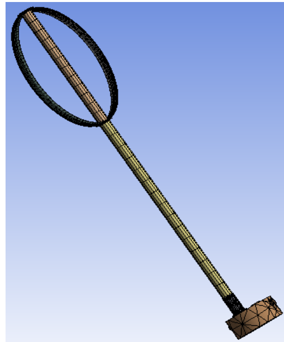
Figure 4 Model of 3 rd configuration (tube, blade and generator) for modal testing
