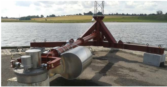
Figure 3 Foundation with concrete feet, generator box and torque arm with air barrels
