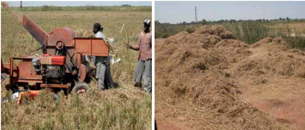
Figure 7.1. Mobile thresher in the field (left) and threshed straw in a pile close to the dike (right) (photo: Ivan Nygaard)
