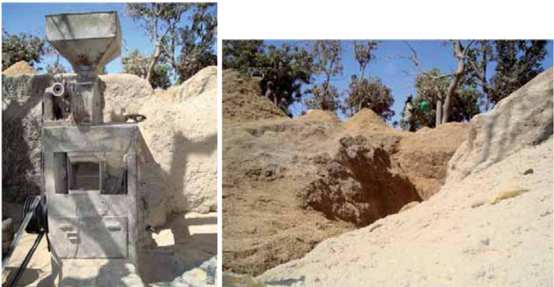
Figure 8.1. Mobile rice huller (left) and pile of rice hulls (right) at the village N4 in Niono (photo: Ivan Nygaard, 2010)
