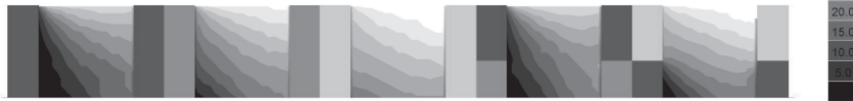
Annual illuminance > 10.000 lux in street canyon. Performed in RADIANCE/DAYSIM (working hours 08-17, Contour range 0-50% in steps of 5%). Weather data., Copenhagen (*DRY)
