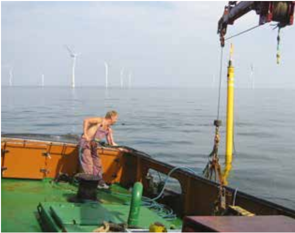
Deployment of acoustic datalogger (POD) outside the Horns Rev Wind Farm. PHOTO: ELSAM A/S
