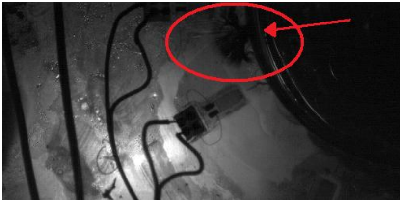
Figure 4: Image from the high-speed camera. The initial fragmentation is marked with the circle and arrow.
