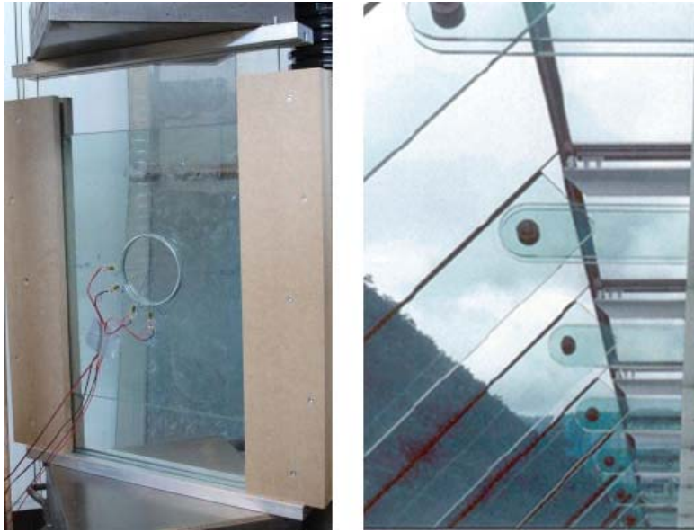
Figure 1: Experimental setup for a glass dowel discs joint (left) and a traditional pinned joint [1] (right).
