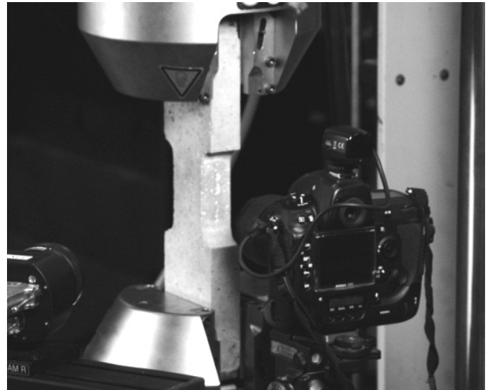
Figure 4: reinforced prism in tensile test setup.
