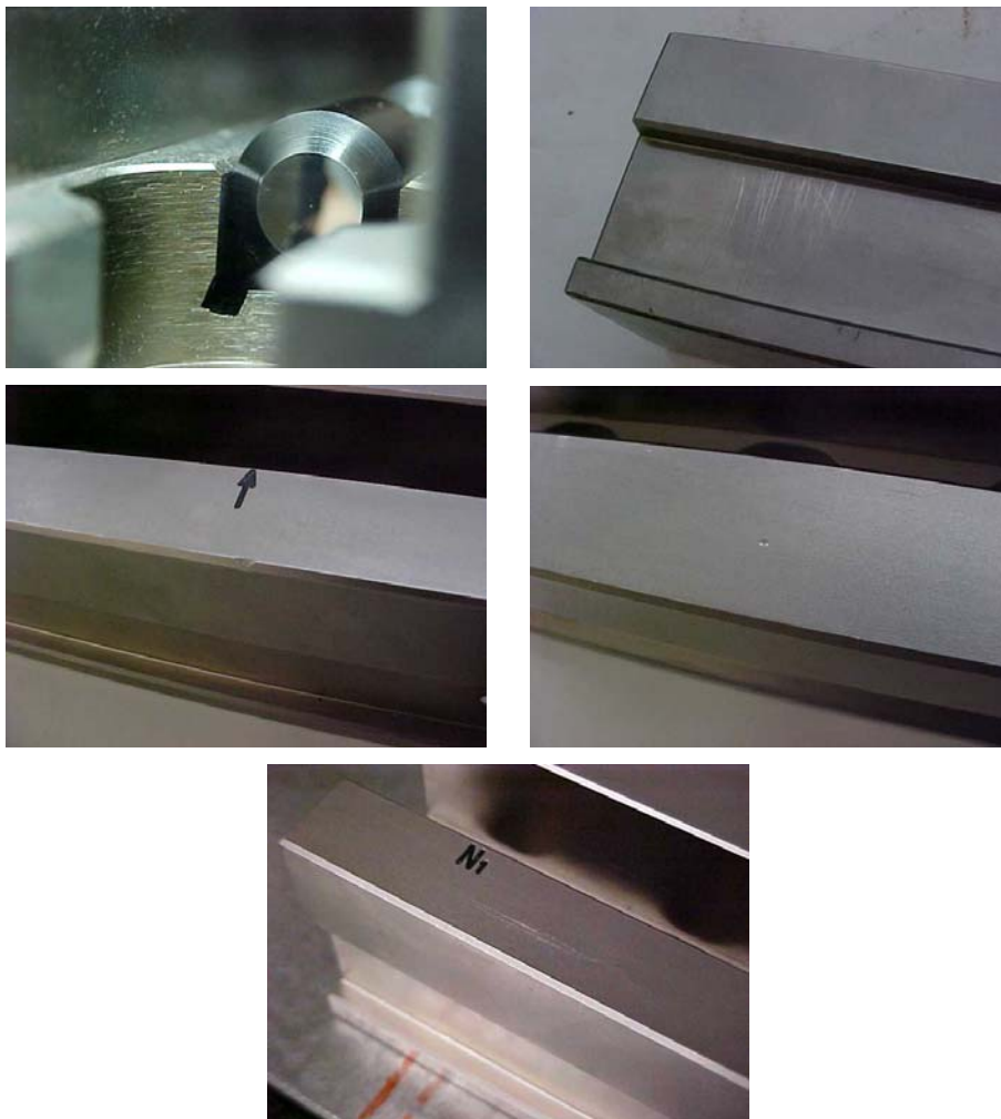
Fig. 4 - Some damages (scratches and points) observed and communicated by INMETRO.
