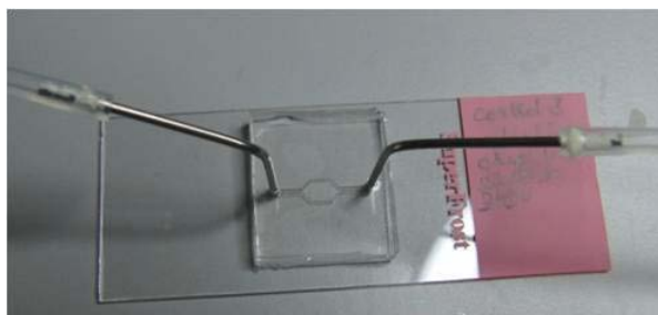
Figure 5.6: Fully assembled microFISH device with interconnects and tubings to connect it to the syringe pump
